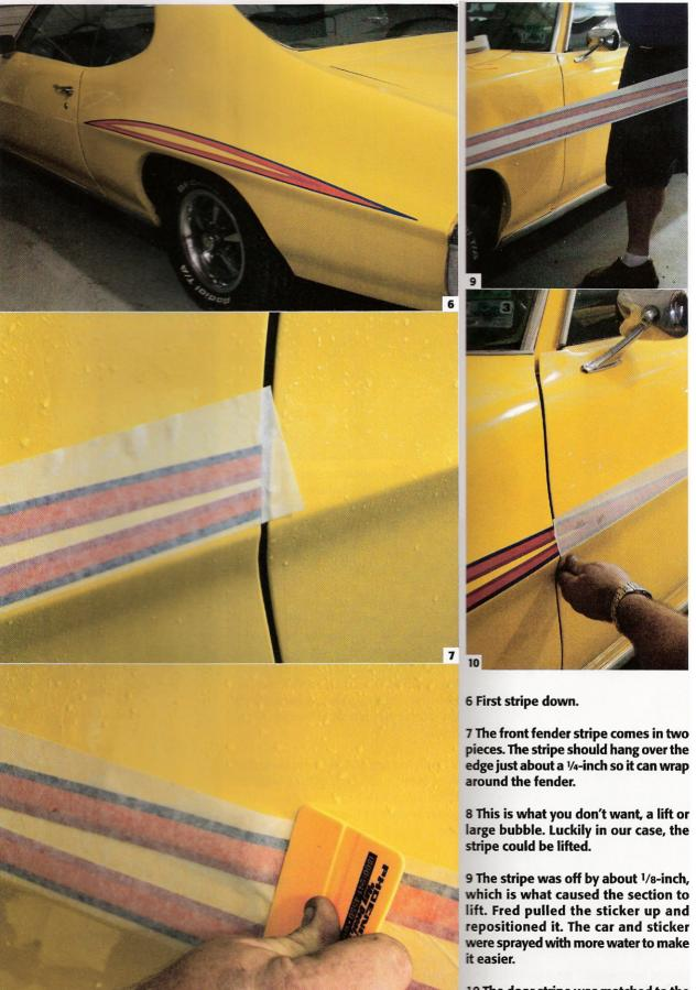
10 The door stripe was matched to the fender and placed on like the rest.
