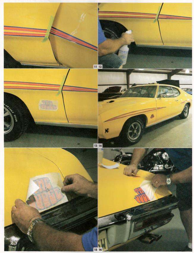
11 The door was opened and the overhang was wrapped around the edge of the fender and taped down with some green painter's tape. This will hold the stripe in place and allow the adhesive to cure and is only required when a short piece is wrapped over an edge.
