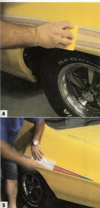
1 The GTO had been washed and wiped down with alcohol before a mixture of soap and water was sprayed on the rear quarter-panel. The soapy water deactivates the adhesive for a short time, which allows the stripe to be positioned on the car.
