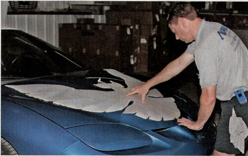
Having laid the decal in the desired location, we use masking tape to mark the intended placement.
