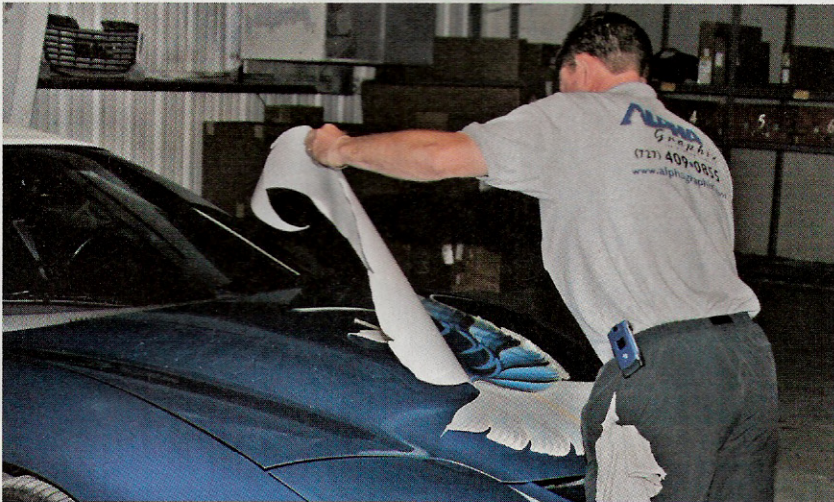
We remove the paper liner, exposing the adhesive side of the decal.
