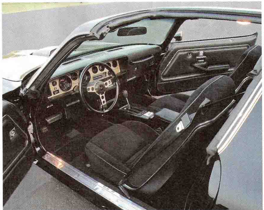
The cabin features the code-19B1 Lombardy custom trim group (velour) upholstery, and the seat covers were re sewn with OEM material. Brian said that it was a nine-month wait for Fryers Upholstery, but the results were well worth it. An inch of additional hushmat-type insulation material was added, as well as package tray and trunk padding.
