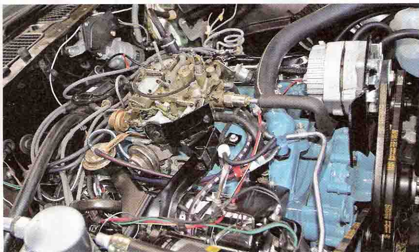
The attention to detail on the engine can be seen much better with the shaker removed. How were all of the vacuum hoses done? Nyle says, "We studied schematics to get the colors and markings for the hoses, and then we hand-painted them. Some are original pieces and others we matched at a local parts store." M&H made new wiring harnesses using the originals as a guide, matching the gauges, colors, and connectors. The belts are not correct. "We can't get GM belts date-coded after 1976," says Nyle. The original No. 17058266 Q-jet was restored and dialed in by Jim McGowan at the Quad Shop.
