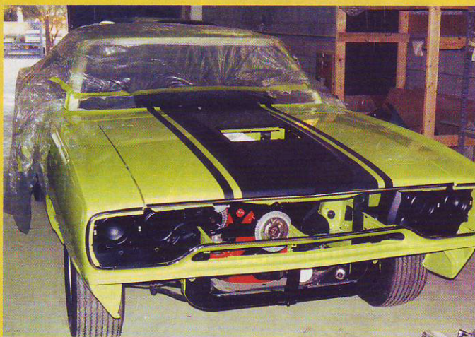
Air Grabber hood was striped before the functioning mechanism was installed; it took three chrome shops to make bumpers perfect
