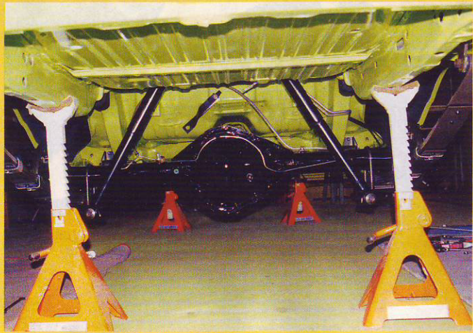
To prevent any undercarriage scratches, jackstands were heavily padded; powdercoated rear axle was test-fitted before installation
