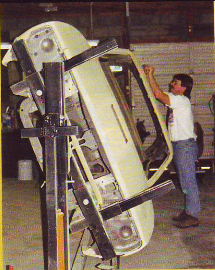
Rotisserie made accessing roof easy while block sanding between coats of DuPont primer
