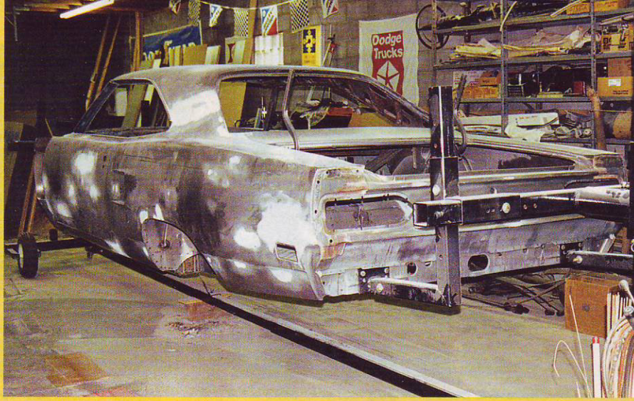
The Road Runner was mounted on a rotisserie after being plastic media blasted, then a thin coat of body filler was applied to level uneven areas
