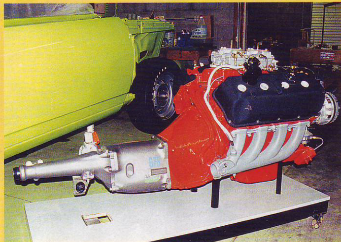
Ready for museum display, the rebuilt 426 Hemi and 18-spline four-speed sat on Rob's homemade engine stand before installation
