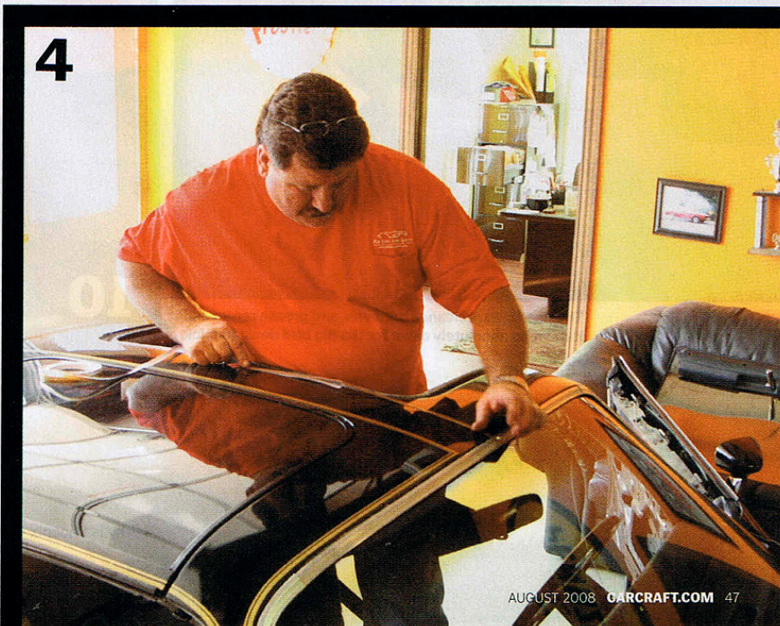
The two parallel stripes that run the length of the car should be spaced approximately 4 inches apart. This spacing needs to be kept from the hood to the roof and on to the trunk lid.
