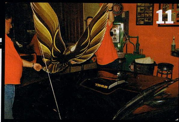
Here is where two people were needed. The backing (not the masking paper) was removed before the decal was transferred to the hood.
