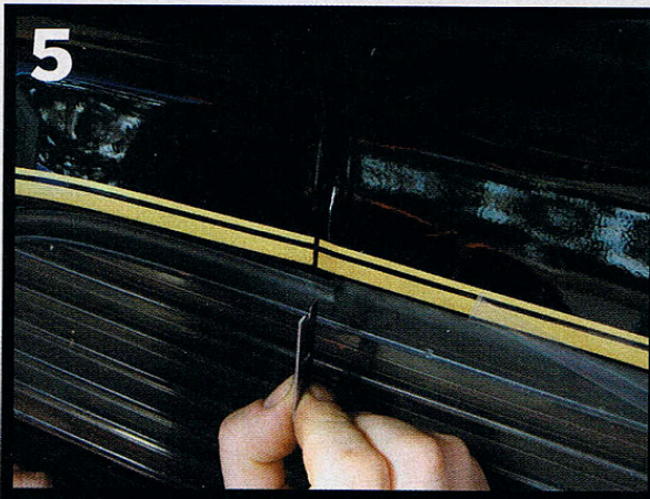
5 The taillight and trunk stripes were laid as one piece and then cut in the center with a razor blade.
