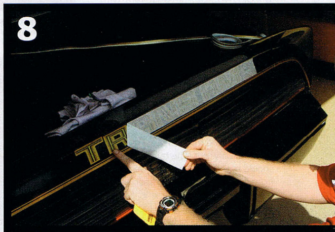
8 After using a squeegee to work the air out, the masking was carefully removed. The vinyl can peel up, so slowly removing the masking works best.
